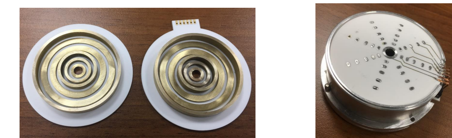
Figure 4 Photo of fabricated RF carpet trap. Left: ring electrodes loaded on ceramic PCB substrate; Right: two piece of RF carpets consist the RF carpet trap.
