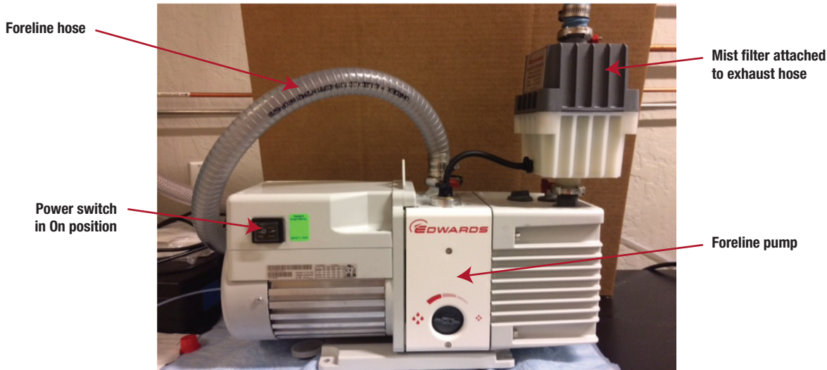
Figure 7. Foreline pump with mist filter
