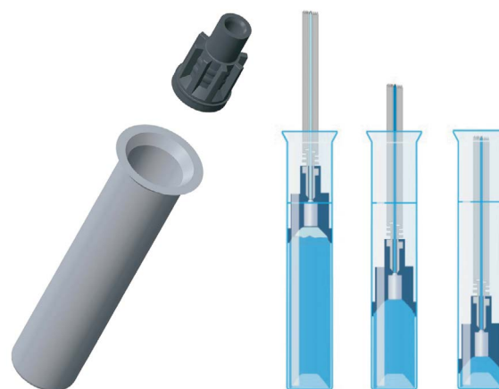
Figure 1. Dionex AS-DV Autosampler sample displacement filtration.
