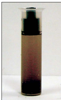
Figure 2. Filter cap inserted into the Dionex AS-DV Autosampler vial. Note heavy sedimentation.
