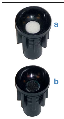
Figure 3. (a) Unused and (b) used filter caps.
