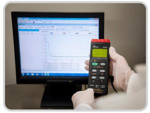
Uploading recorded data from 4-channel datalogger with Type K thermocouples
