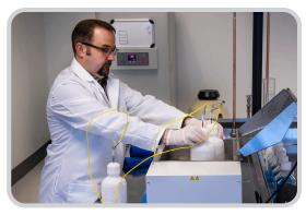
Placing bottles in 37°C preheated recirculating water bath
