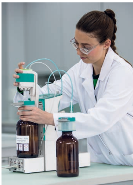
Fig. 1: Due to the Liquid Adapter, users do not have to open reagent bottles and benefit from full traceability of their titrations.
