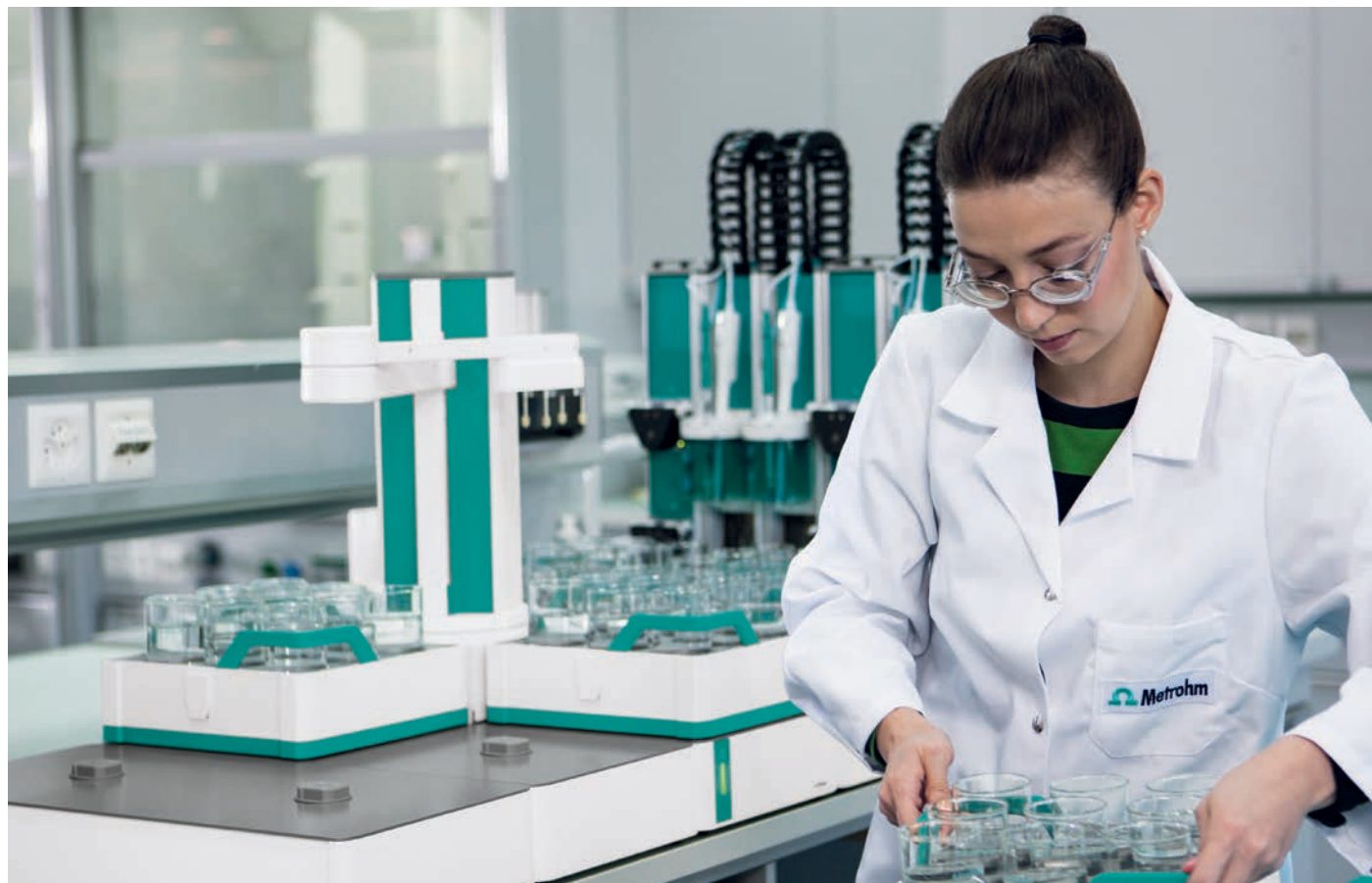
Fig. 2: The Omnis Sample Robot accommodates up to 175 samples and enables the exchange of racks with already analyzed samples while the system keeps analyzing.
