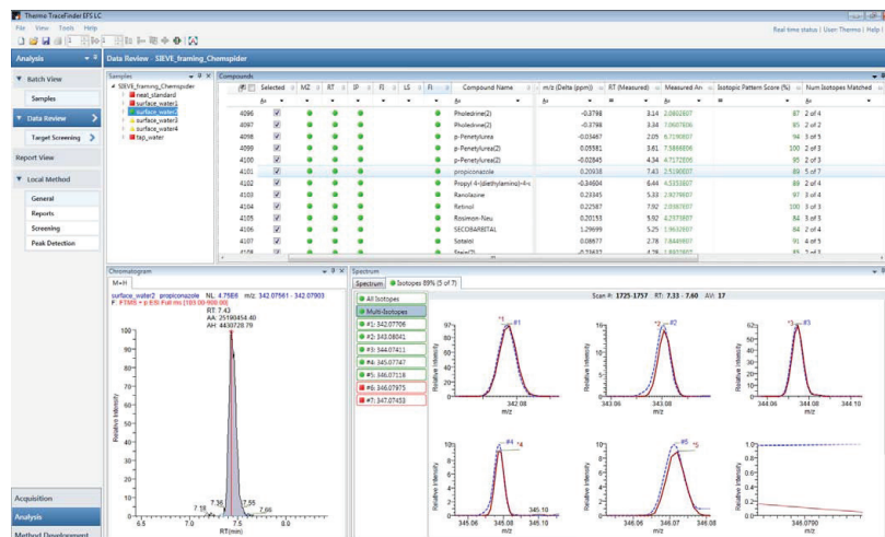
FIGURE 7. Confirmation of the unknown screening results from SIEVE software, propiconazole taken as an example: the extracted ion chromatogram at the determined retention time gives a clear signal free from interferences, the isotope pattern match shows close to perfect overlay
