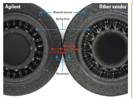
Photomicrographs of pump piston seal from Agilent and other vendor
