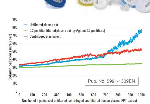
Unfiltered, centrifuged, and filtered plasma extracts Zorbax RRHD Eclipse Plus C18, 2.1 x 50 mm, 1.8  $\mu m$  column, PN 959757-902
