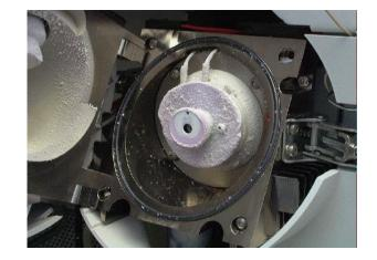
Salt build-up in LC-MS ion source from unextracted salts ESI Ion Source contamination after 3000x Urine Dilute/Shoot Injections
