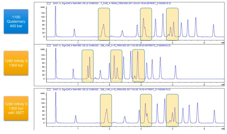
2.1x100 mm Zorbax Eclipse Plus, 1.8 µm column; Flow = 0.8 mL/min
