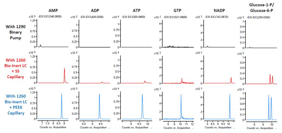
Column used was 2.1 x 100 mm, 2.7 µm Agilent InfinityLab Poroshell 120 HILIC-Z (PEEK lined stainless steel); A: 10 mM Ammonium Formate pH 6.8 in water, B: acetonitrile + 10 mM Ammonium Formate pH 6.8, 95-30% B in 10 minutes, 0.25 mL/min, 0.2 µL injection (5 ng each on column), MS Source: ESI-, m/z 191.02, 346.06, 426.02, 505.99, 521.99, 742.067, 743.067, 259.03
