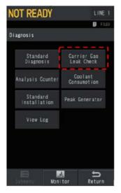
If the leak check fails, please check your gas plumbing, inlet top and column connections. You must resolve the leak issue before proceeding.
