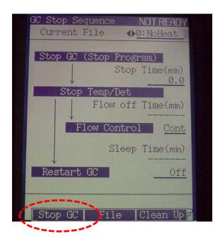
c) From GC-2030 front panel: press the home button open the menu and "stop GC" to stop the system.
