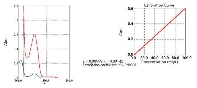
The figure on the left shows the absorption spectrum of detergent A. The sample concentrations are 100 mg/L (red) and 10 mg/L (blue). The figure on the right shows the calibration curve at a measurement wavelength of 225 nm. These results illustrate the method of calculating quantitation limits based on measurements conducted using an UV-Vis spectrophotometer.
