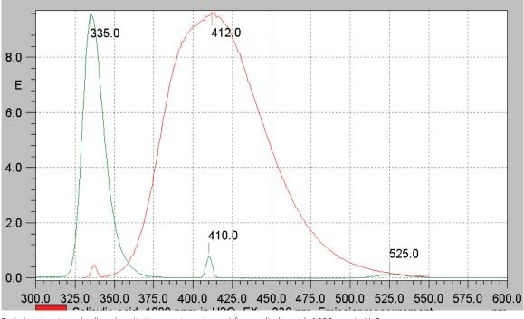
Emission spectrum (red) and excitation spectrum (green) from salicylic acid, 1000ppm in H<sub>2</sub>O
