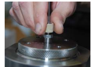
Vessel connector attaches to closure nut.
