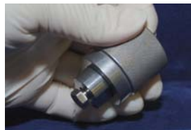
Endcap goes into Closure nut.
