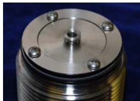
Screws secure seal cover.
