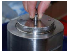
Apply PTFE Tape to adapter fitting 1/8" FNPT to 10-32 THD and attach to cover. (Not necessary to remove every use.)
