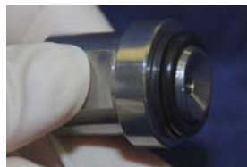
Back-up ring and O-ring fit onto end cap.
