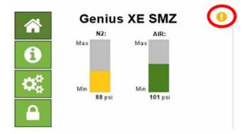
Toggle the warning indicator in the top right corner of the HMI to view warning code.
