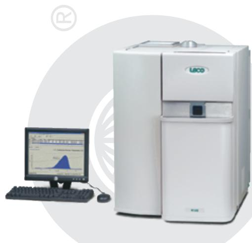
The LECO RC612 is a multiphase carbon and moisture determinator specifically designed to differentiate different forms of carbon by the temperature at which they oxidize. This capability facilitates the determination of the amount of carbon present on the surface of steel sheets or rods, which is relative to the amount of oils or carbonaceous materials. The LECO RC612 provides a robust, fast, and direct determination with little to no sample preparation required.
