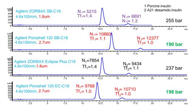
In these chromatograms the Poroshell 120 SB-C18 2.7um column provides 2X the efficiency of the 80Å SB-C18 1.8µm. This is due to the larger pore size and more rapid diffusion in the 120Å pores. Switching from the ZORBAX Eclipse Plus C18 to Poroshell 120 EC-C18 also provided an increase in efficiency with the change from 95Å to 120Å pore size. In addition, the peak shape of insulin on both Poroshell 120 columns was improved with greater access to the pores.
