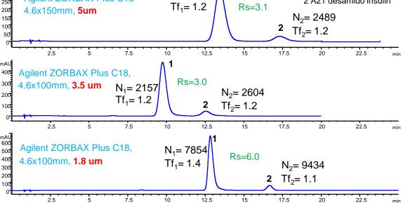
The insulin method was run on 5 µm, 3.5 µm, and 1.8 µm Agilent ZORBAX SB-C18 columns and Agilent ZORBAX Eclipse Plus C18 columns. The data demonstrate improved efficiency using the smaller 1.8 µm particle columns. While these columns are not the ideal pore size columns, efficiency should still be expected to improve with smaller particle sizes, as it does here with insulin.
