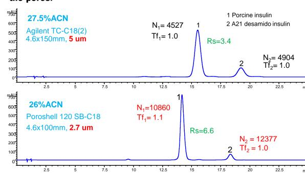
In addition, the Poroshell 120 column provides higher efficiency than the 5um Agilent TC-C18 (2). The chromatogram shown on the TC-C18 (2) column is the one run with 27.5% organic in the mobile phase so that the retention times could be more closely matched. The improvement in the efficiency when comparing these two columns is due to the benefit of the smaller particle size with a larger pore size.
