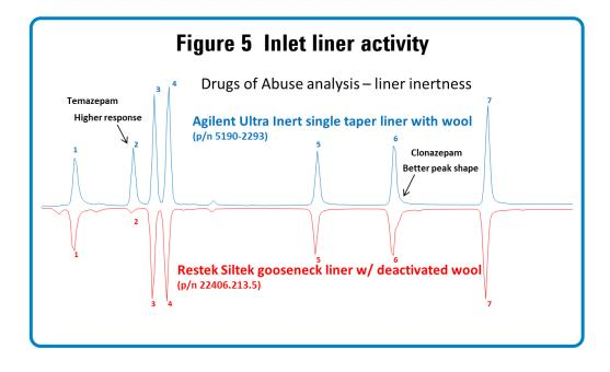
For other links in the flow path chain, protocols were developed using trace levels of the same labile compounds. Side by side comparisons were made, alternating between passivated and standard components. All other test conditions were kept constant to provide as fair a comparison as possible.
