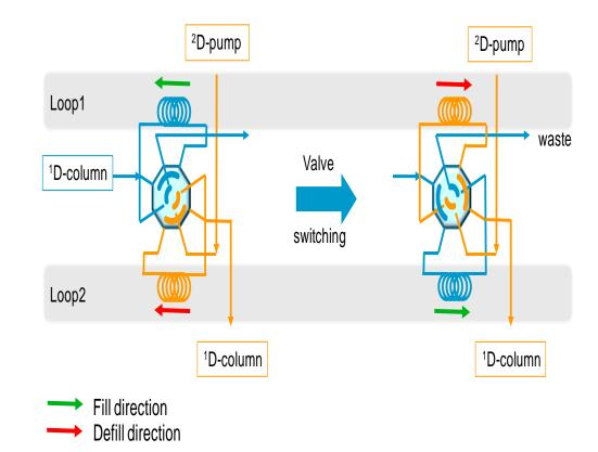
All flow paths are equal (no additional bridging loops) Symmetric contercurrent fill/defill of loops (reducing band-spread All in one valve (no synchronization, costs)
