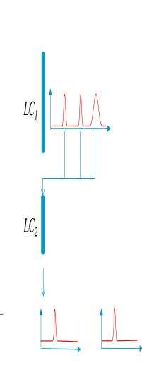
Only **parts** of the effluent of the first column – the peaks eluted from the 1st dimension column - will be injected to the second column. Typically a peak from the first dimension will be samples as a whole and a gradient with a longer run time than the collection time will be used. Also longer columns with higher seperation efficiency are being used in as 2nd dimension column.
