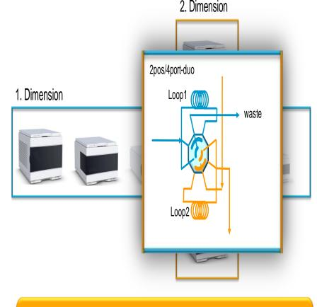
New Agilent-only special 2D-LC-valve. Single valve with fully symmetr low-paths and symmetric fill/flush-out behavior. Only valve that allow countercurrent flush-out of loops.
