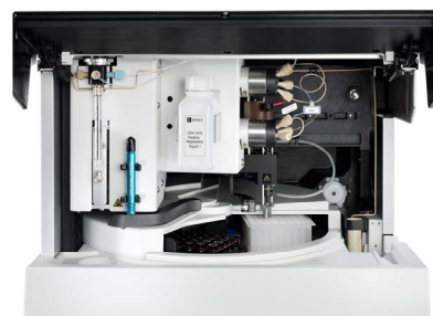
Figure 20. The UltiMate 3000 Semipreparative Autosampler provides large volume injections up to 2.5 mL.
