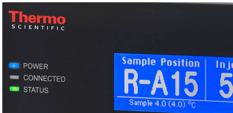
Figure 7: Sample thermostating down to 4 °C ensures sample integrity.
