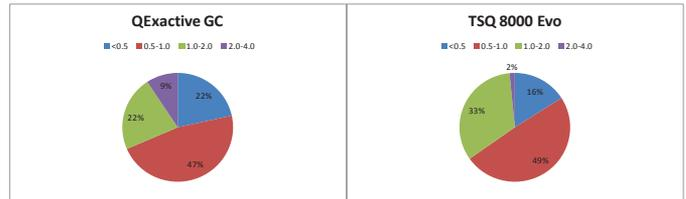
**FIGURE 4.** Comparison of the IDL<sub>99</sub> (ng/g) calculated for 132 pesticides from a 5 ng/g matrix-matched standard from the Q Exactive GC system (left) and TSQ 8000 Evo triple quadrupole GC-MS (right). Percentage of pesticides and corresponding IDL interval relative to the total number of target compounds (132) is indicated.
