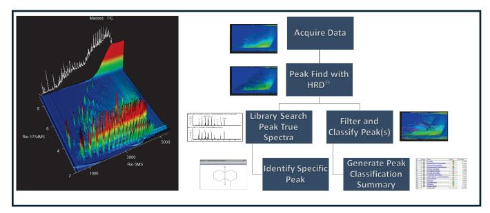
Figure 1. Total Ion Chromatogram Plots of Heavy Fuel Oil Sample: 3D Surface plot of El acquisition is shown on the left with the white reconstructed chromatogram in the background showing what a single dimension separation would have looked like. The data interrogation workflow for the combination of GCxGC and HRTOFMS data is shown on the right.
