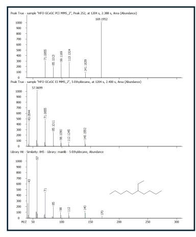
Table 2. Major fragments of 5-ethyldecane peak from the PCI spectra with calculated mass accuracies shown.
