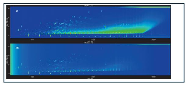
Figure 4. Comparison of full TIC chromatogram of heavy fuel oil acquired in EI and PCI modes, illustrating the excellent retention time correlation between acquisitions where no manual hardware intervention or venting was required.
