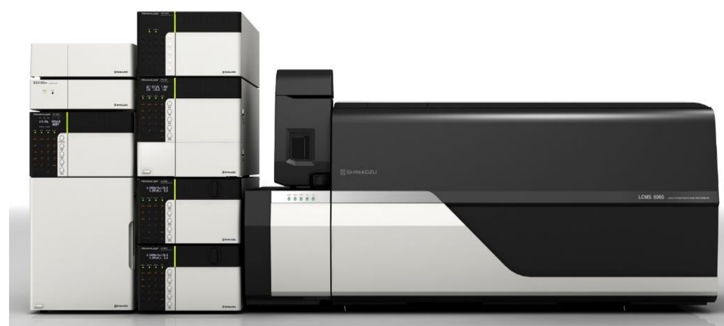
LCMS-8060 5 msec polarity switching, 30,000 u/sec scanning speed, MRM monitoring
