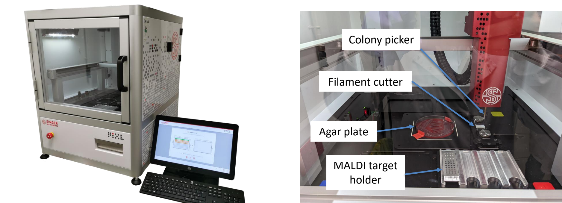
Figure 1. (Left) PIXL colony picking robot and (right) internal layout showing colony picker tip, filament cutter, target holder and agar plate.
