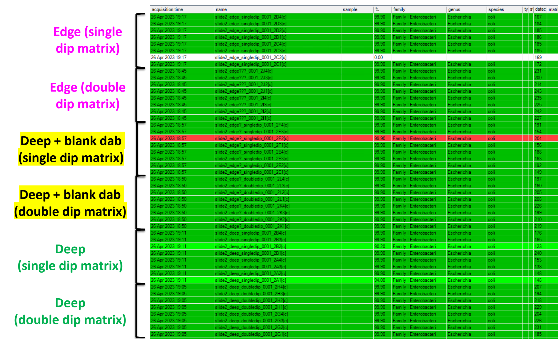
Figure 4. SARAMIS results for E.coli samples prepared using Method C i.e. automated smear deposition and automated single or double dip matrix deposition. Dark green = >99.9% confidence, light green = 90.0 – 99.8% confidence, red = mixed ID, white = no ID.
