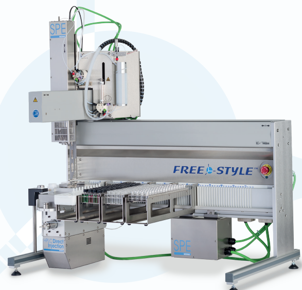
Robotic system FREESTYLE for new automated QuEChERS method
