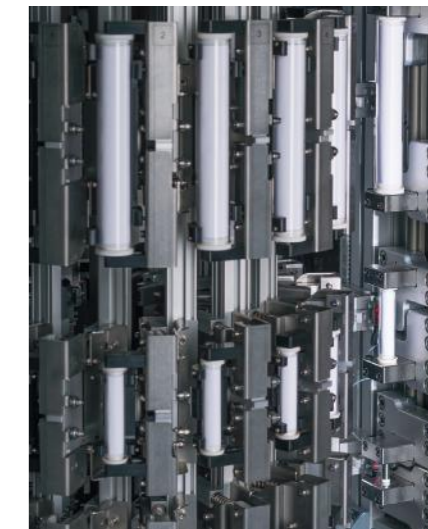
Column carousel is in the rear position with locked columns in the column tower.
