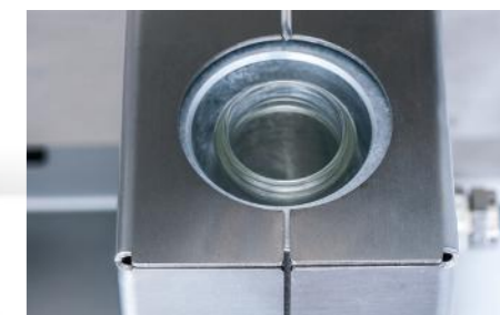
Heating from sample vial via the sample loop and tubing to the first column.
