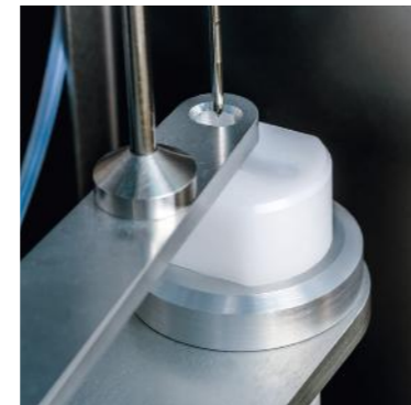
Rinsing port for cleaning the needle inside and outside
