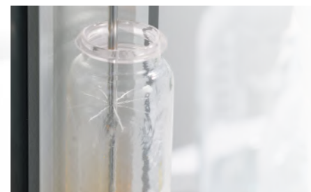
Rinsing of sample vial for quantitative transfer
