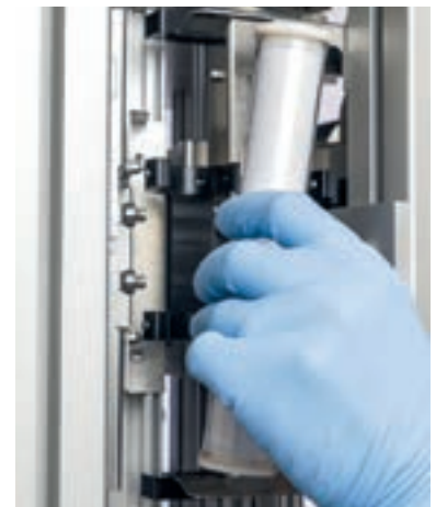
Insert the ready-to-use columns in the carousel and press „Start“.
