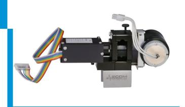
The unit is supplied with AMY17 PCB board of dimensions 100 x 160 mm (3.94 x 6.30 in) .It powers the lamp and control the unit.
