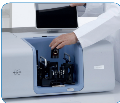
Sufficient space, even for bulky accessories in QuickLock™ mount with lock and release button in front.
