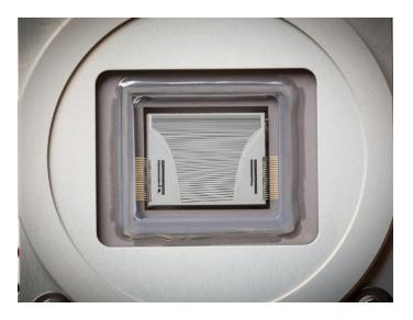
**Figure 7.** The detector is hermetically sealed, so an argon purge is not required when measuring UV wavelengths. The seal also extends the detector lifetime.
