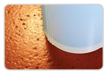
Figure 4. Competitive Hotplate Image Showing Deep Pores in the Surface
