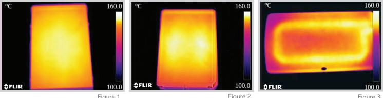
Figure 1. Thermal Image of Savillex HPX-100 Hotplate
