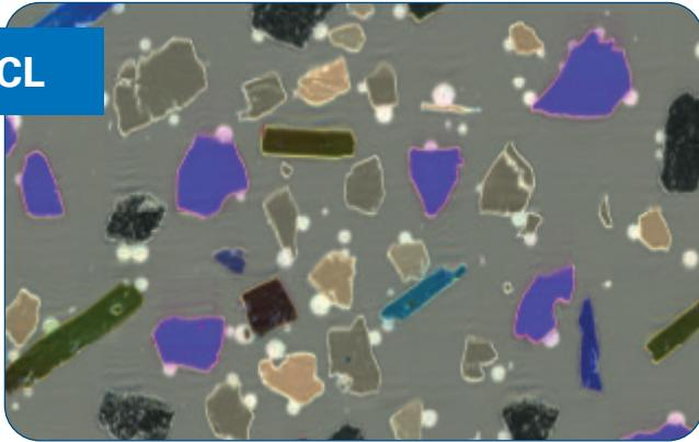
Infrared laser imaging readily evaluates minerals and geochemical properties. The example above shows the differentiation of various oxide minerals based on their reflectance properties.
