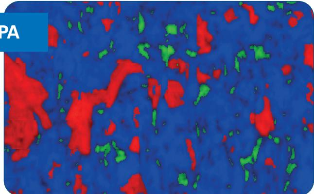
Composition, thickness and homogeneity of this polymeric material is easily assessed by  $\mu$ -FT-IR. False-color image shows: POM (blue), PTFE (green) and Aramide (red).
