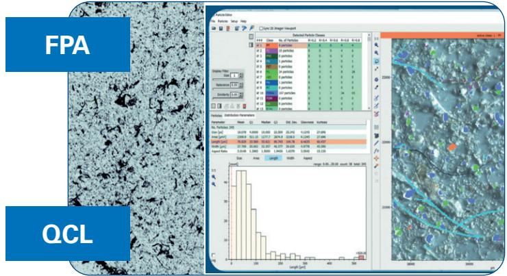
FT-IR imaging is the gold standard in microplastics analysis but IR laser imaging is catching up fast. Left: IR laser image; Right: automated microplastics analysis.
