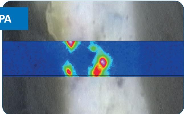
Determining the ingredients of a mixture has never been so easy. In this case, a pharmaceutical pellet was analyzed for impurities. The impurity (red) stands out clearly from the API matrix (blue).
