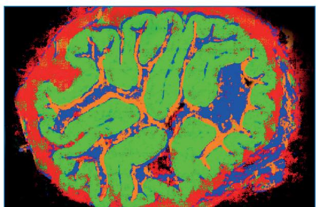
Localize different components and points of interest of your sample completely automated. The above image shows the Result of k-means cluster algorithm of an FT-IR Image with 2 million spectra. Everything was determined automatically within around 10 seconds.
