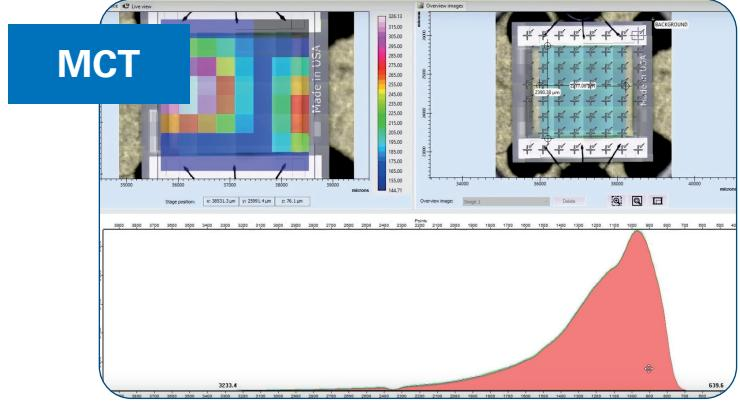
The quality and emission behavior of IR emitters (e.g. voxels or LEDs) can be checked by  $\mu$ -FT-IR. The above picture shows an inhomogeneous radiation distribution of an LED.
