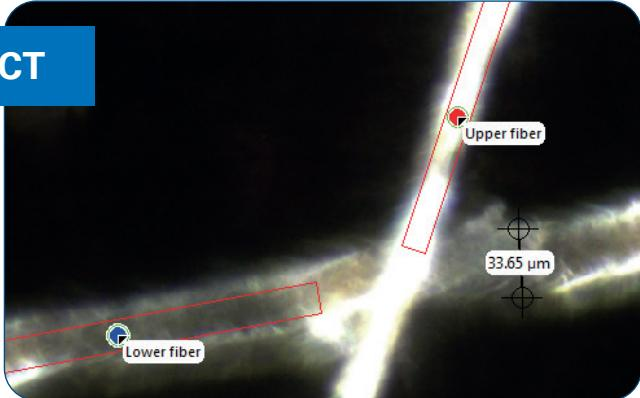
IR microscopy is an outstanding tool for forensic science. In this case, fibers were examined to obtain clear evidence of their origin. Knife-edge apertures ensured optimal spectral quality.
