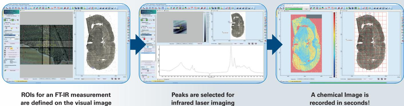
**Note:** This process can also be turned around: IR Laser Imaging is used to prescreen a sample quickly and only collect FT-IR spectra at selected regions of interest.
