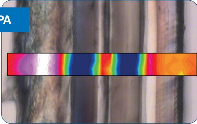
IR imaging makes it easy to analyze laminates and multilayer structures. This multilayer paint chip was examined using high-resolution ATR imaging to determine the cause of a car accident.
