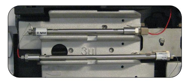
Custom length columns (>15 cm) can be created by joining together using a 0.12 x 70 mm tube (PN G1316-87303). This tube only adds 0.79  $\mu$ L volume and allows for a straightforward arrangement of the columns within the G1316 column heating compartment.
