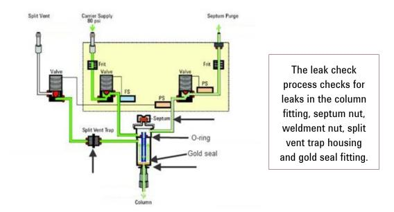
If the leak remains, do basic inlet maintenance: replace the septa, liner and o-ring (demos available at <a href="http://www.agilent.com/chem/gcinletcare">www.agilent.com/chem/gcinletcare</a>)
