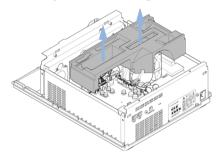
Break out the metal piece from the middle of the front of the Z-Plane (this leaves a circular hole).
