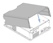
12 Lower the cover into place. Ensure the clips snaps firmly.
