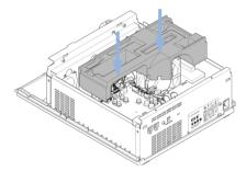
**9** Engage the slots on the top plate onto the Z-Plane.
