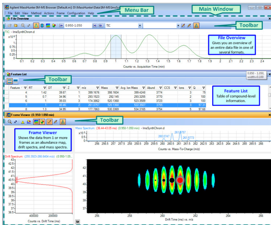
Figure 1 The main functional areas of IM-MS Browser after IMFE is executed and a frame extracted. You can also calculate Collision Cross Section as shown in Figure 2 on page 17.
