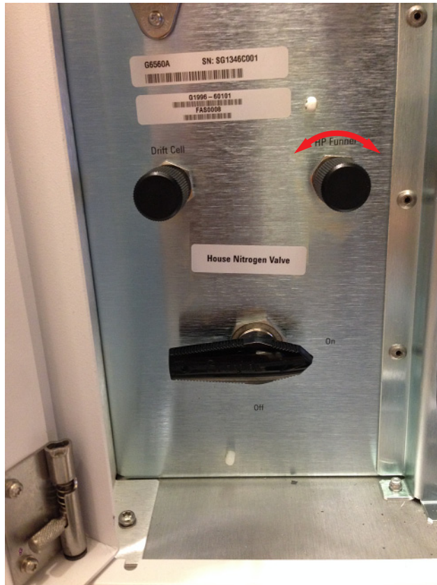
Figure 8 Adjusting the High Pressure Funnel pressure regulator
