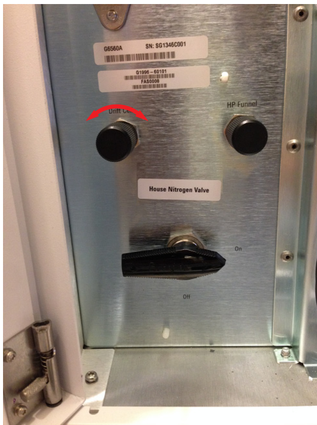
Figure 10 Adjusting the Drift Cell pressure regulator
