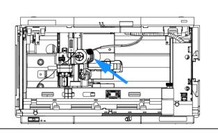
3 Unplug the inlet / waste tubing assembly from the bolt carrier (located on the top center of the front cover) by moving the snapper as indicated by the arrows. Slide the tubings out to the bottom.
