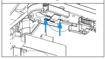
**5** Slide the tubing through the hole in the needle carrier assembly (from bottom to top) and out of the holder in the z-arm assembly.
