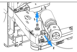
7 Using the 4 mm wrench and the 5/16" wrench for counter-holding connect the valve to needle tubing to the needle. (Viewed from the bottom)
