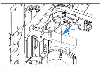
6 Install the new valve to needle tubing assembly by clipping it in to the holder in the z-arm assembly (1) Important!!!), slide it through the hole in the z-arm (2) and out on the bottom of the needle carrier assembly (top to bottom). Screw the finger-tight fitting into the port of the diverter valve (3).
