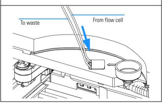
6 Connect the finger-tight fittings of the inlet / waste tubing assembly to the ports of the diverter valve.
