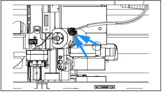
1 Locate the diverter valve with the finger-tight fittings of the inlet / waste tubing assembly (the figure shows the open fraction collector seen from the front).
