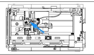
**2** Unscrew the finger-tight fitting of the valve to needle tubing assembly at the diverter valve.
