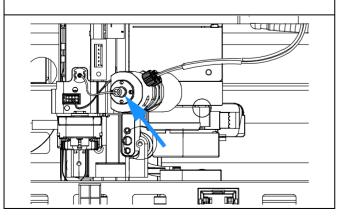
**3** Using the 4 mm wrench and the 5/16" wrench for counter-holding unscrew the valve to needle tubing from the needle. (Viewed from the bottom)
