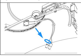
7 A color coded ring on one of the tubings and the valve body indicates, which cable belongs to which port. IMPORTANT: It is absolutely vital to connect these tubings as described, in order to maximize their lifetime and operating security.
