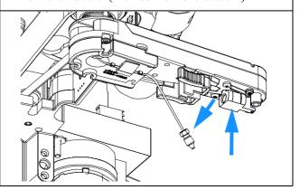
**4** Un-clip the tubing from the bottom of the needle carrier assembly.
