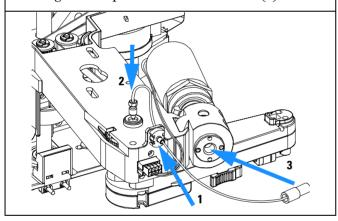
8 IMPORTANT: After fixing the screw clip the tubing into the guide on the bottom of the needle carrier assembly. IMPORTANT: It is absolutely vital that the tubing is installed as described, to maximize the lifetime of the tubing.
