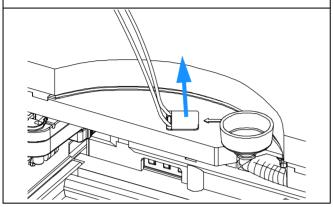
**5** The rear tubing (with the label with the arrow) must be connected to the flow cell of the detector. The front tubing must be inserted into the waste container.
