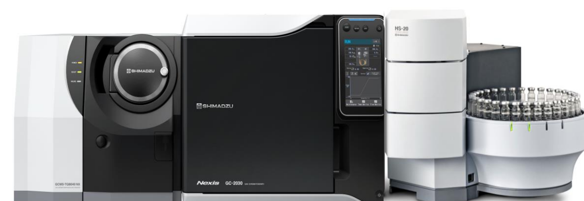
Figure 2 GCMS triple quadrupole mass spectrometer with headspace autosampler
