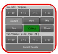
During the separation *Run* (or *Extended Run*) some buttons will be disabled or hidden. Some more complex operations are allowed only in *Pause* (or *Extended Pause*) state (e.g. Gradient, Detection...).
