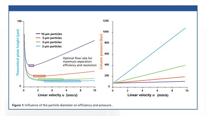
Reducing the particle size, however, dramatically increases column back pressure (Figure 1, right), which presents a challenge in the design of chromatography systems that can operate reliably at higher pressures.
