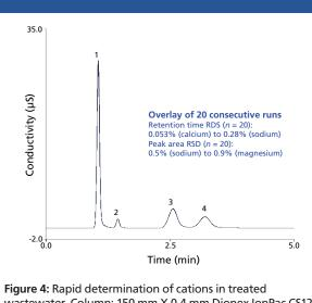
wastewater. Column: 150 mm X 0.4 mm Dionex IonPac CS12A-5µm; eluent source: Dionex EGC-MSA capillary cartridge; eluent: 28 mM MSA; flow rate: 18 µL/min; temperature: 30 °C; suppressor: electrolytic capillary anion suppressor; sample: treated wastewater (1:10 dilution). Peaks: 1 = sodium (19.6 mg/L), 2 = potassium (0.8 mg/L), 3 = magnesium (3.5 mg/L), 4 = calcium (3.1 mg/L).
