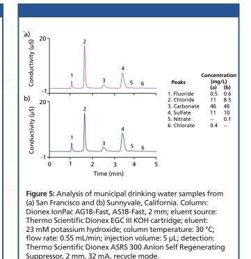
capacity to maintain resolution even in a short-column format, as shown here. When the short column is packed with smallerparticle resin, back pressures produced at higher flow rates are reduced and shorter overall run times can be achieved. Anions can be determined with high resolution even in drinking, surface, groundwater, and wastewater matrices, all in less than 5 min.
