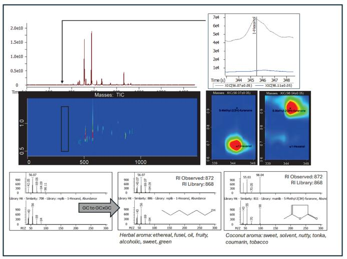
Two analytes, 1-hexanol and 5-methyl-2(3H)-furanone, coelute in a GC-TOFMS separation of basil. These analytes appeared together as one peak with a combined spectrum. The enhanced peak capacity of GCxGC chromatographically separated these compounds in the second dimension, improving the similarity score for 1-hexanol and revealing the previously obscured furanone. Both analytes have interesting aroma properties that may contribute to the aroma profile of the basil.
