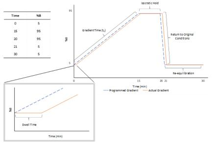
*Figure 1* Schematic of the programmed gradient, with the corresponding gradient timetable and the actual gradient
