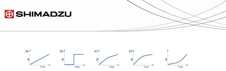
Figure 2 Schematics of different gradient profiles; (A) linear, (B) step, (C) segmented and (D) curved profiles
