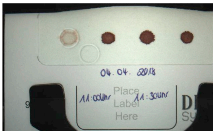
Figure 5. Picture taken by the built-in DBS-A camera showing a typical HemaXis DB blood spot card after analysis of spot 1.
