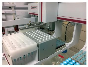
Figure 1. MPS robotic<sup>PRO</sup> sampler with the GERSTEL Fast Filtration Option.
