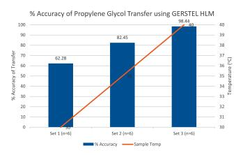
Figure 2. % Accuracy of propylene glycol transfer using the GERSTEL Heated Liquid Syringe Module.
