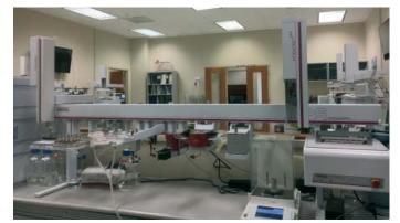
Figure 1. MPS robotic/robotic<sup>PRO</sup> sampler configured with GERSTEL automated sample preparation options.
