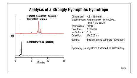
Hydrotropes are used to improve surfactant formulations. The weak anion-exchange properties of the Acclaim Surfactant column improve hydrotrope retention and resolution compared to purely reversed-phase columns.
