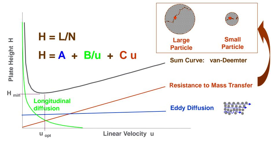
The smaller the plate height, the higher the plate number and the greater the chromatographic resolution
