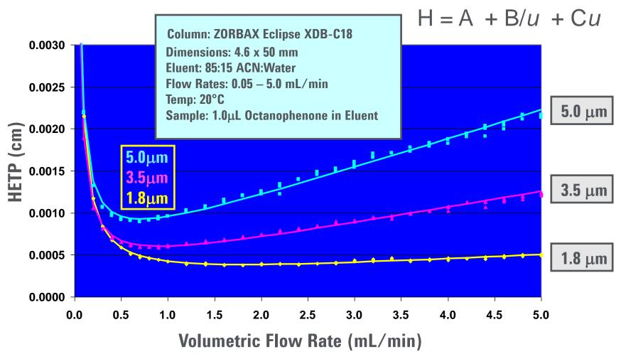
Smaller particle sizes yield flatter curves, minima shift to higher flow rates
