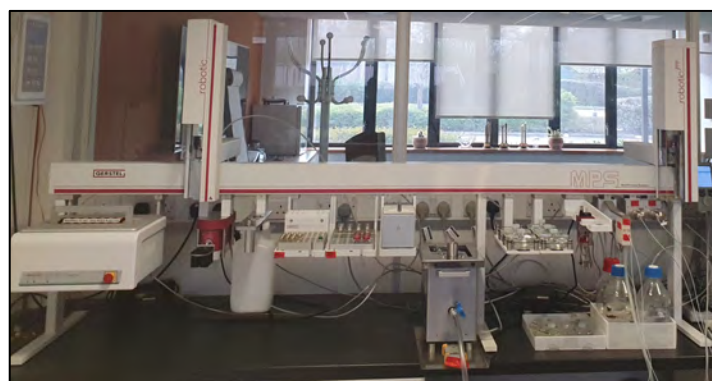
Figure 2: Automated sample prep configuration for the analysis of nitrosamines in API and drug products
