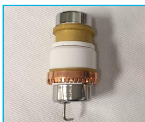
Figure 2. Agilent GC/MSD TAD 1 Electron Multiplier.
