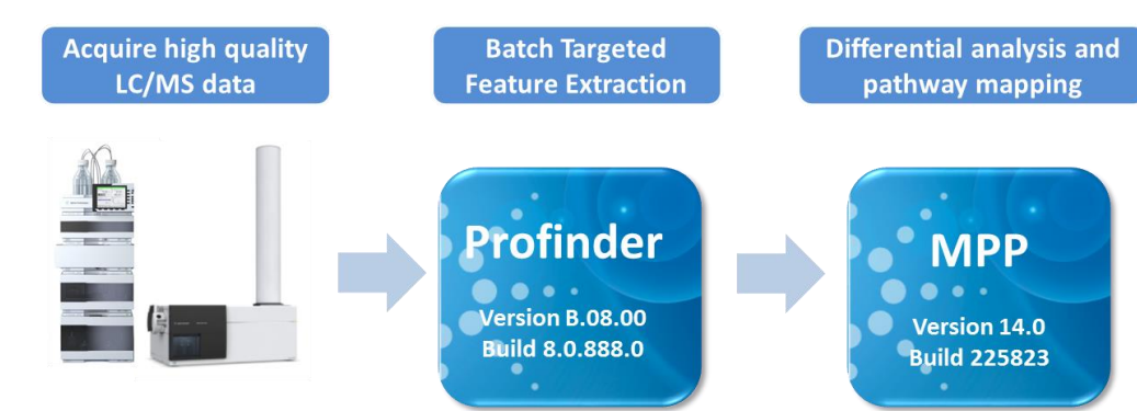
Figure 1. LC/MS metabolomics workflow for high quality data acquisition and analyses.
