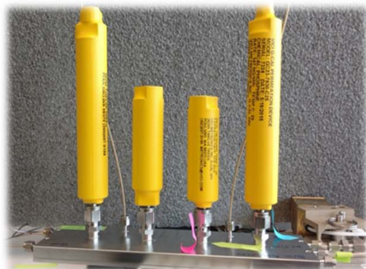
Figure 4. Permeation tubes of 4 calibrants in the dilution block.
