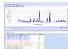
FIGURE 5. SIEVE software results after filtering and grouping isotopes. A 'Ratio of Prod/Std' <1 means that component is more abundant in the bench-scale synthesis (or standard) than in the pilot production synthesis. A 'Ratio of Prod/Std' >2 means the component is more abundant in the pilot production synthesis.
