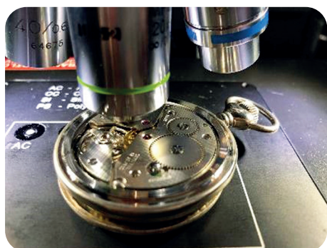
Figure 1: Clock without cover glass under the 20x objective on the SENTERRA II sample stage. Cover glass was removed to improve visual inspection.
